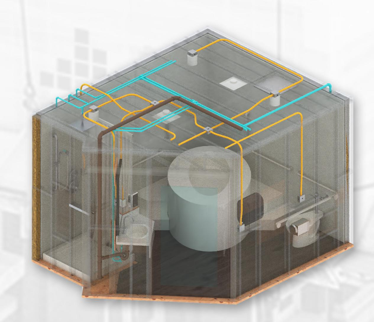
Bathroom Pods are an innovative and efficient construction method well-suited for various projects. Whether you're building a new home, renovating an existing space, or working on a commercial construction project, this technique can help you save time, money, and resources while achieving high quality and consistency!
